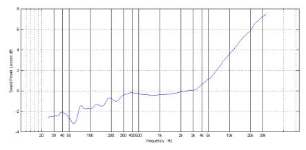
This is how the hall equalizer FR should be to create a flat Sound Power Density Frequency Response in the Benedum center from the sound source (loudspeakers) with a flat Sound Power Frequency Response.
