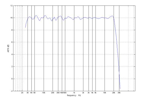
Now is the time to apply phase/delay correction based on DFR. The TDA graph after both equalizations
