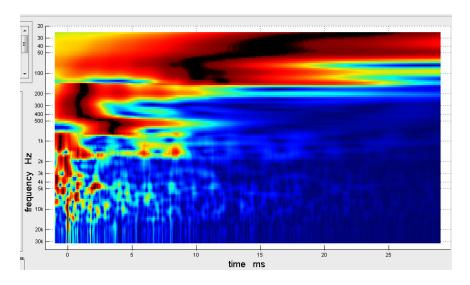
The maximum of the detector's output signal represents not only time of arrival but also the magnitude (power) of the arriving frequency components. And as this magnitude represents one particular moment in time, it is in a way free of interference (not absolutely) from the delayed signal (reflection) that can be seen later on the graph time axes.
