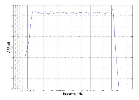
If a loudspeaker system is 3- or 4-way it is a challenge to keep the crossover circuitry well tuned. It is easy to make serious mistakes if you are doing this "blind". This happened with a large (and expensive) 3-way studio monitor where incorrect design decisions introduced a 20 ms delay in an LF band that should not have been in a loudspeaker intended to work as a studio monitor. Let's look at that example.
